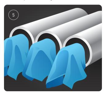
**6.** Just before installing the bearing, wipe clean the shaft where the inner ring will be seated, and wipe clean the housing surface where the outer ring will be mounted.
