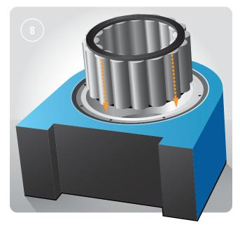
9. Lubricate the rollers using the same oil or grease used on your caster. There is no need to remove the anti-rust coating on the bearing. Rotate the roller assembly one revolution to distribute the lubricant. Center the cage and roller assembly in the outer ring.
