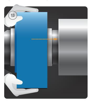
14. Rock the housing back and forth in the direction of rotation to check for bearing freedom of motion. If the bearing binds or cannot move freely, remove the bearing and diagnose the problem. Do not put the roll in service until you can verify that the bearing rotates freely on the roll.
