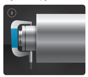
4. Measure the inside diameter of the housing. Take measurements in one direction, and then rotate the micrometer 90 degrees to ensure that the housing is both symmetrical and the proper size. The correct dimensions are shown in the Suggested Fitting Practice Table on page 15.
