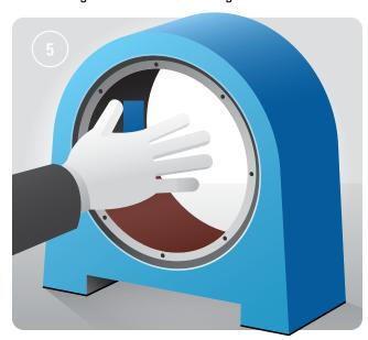
**6.** Remove the roller assembly from the outer ring prior to assembling the outer ring in the housing. The roller-retainer assembly and outer ring are matched and the roller-retainer must be kept together during mounting process. Place the bearing outer ring (without the roller assembly) into the housing and slide it into place. The outer ring is typically a loose fit and easily mounts in the housing. If needed, use
