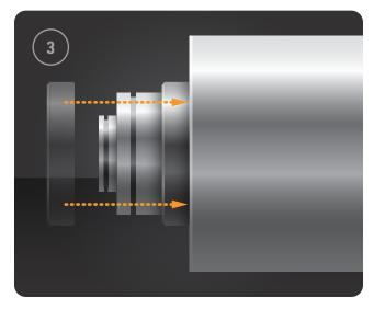
**4.** Install the bearing inner ring on the end of the roll using the same technique and temperature used for the spacer. The inner ring must be firmly seated against the spacer.
