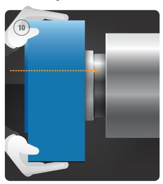
11. Install the end plate on the end of the roll to secure the bearing inner ring in place. Secure the end plate using the appropriate fasteners, further secure with a locking fluid (e.g. Loctite 243). Torque the fasteners as specified by the roll manufacturer.
