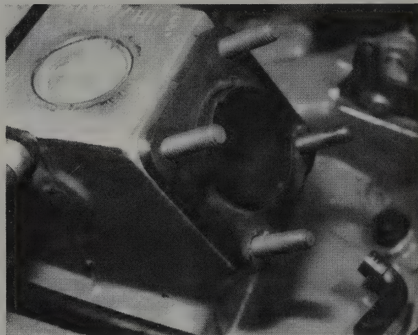
5.44 Carburettor mounting flange liner and gasket
