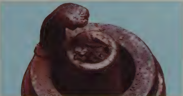
Electrode damage. Electrodes burned away; core nose has been burned, glazed appearance. Fault: initial pre-ignition. Check: as for 'Overheating' but may be more severe. Discard plugs and remedy fault before piston or valve damage occurs
