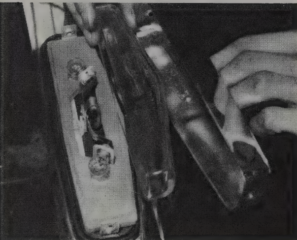
37.1 Removing number plate lamp cover
