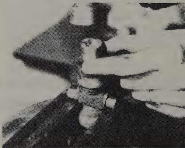
4.5 Using a socket to tap home a bearing cup
