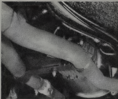
5.47b Exhaust centre mounting
