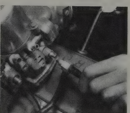
5.41 Uncoupling fuel feed and overspill pipes
