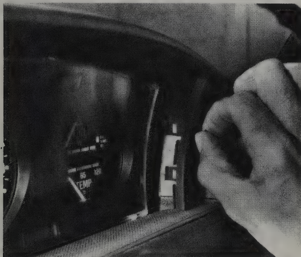
45.2 Detaching instrument panel finisher
