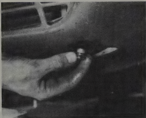
2.3 Removing the radiator drain plug
