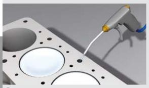
**5.** Clean the bolt hole threads, and remove any contamination, oil and water, e.g. with a blast of compressed air.
