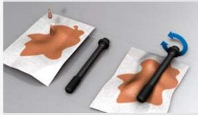
**9.** Lightly lubricate the bolt thread and the bottom of the bolt head by applying a small quantity of oil to a rag and rotating the bolt in the oily rag.
