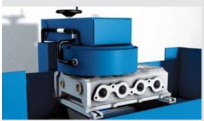
**3.** Remove any gouging, component distortions, grooves or scores, e.g. by surface grinding in a specialist workshop.
