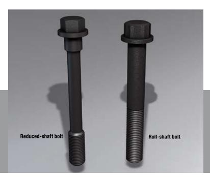
Advantage of stretch bolt: As opposed to a rolled shank bolt, it can be tightened beyond its elastic limit (yield point) into the plastic region – a guarantee for high and uniform bolt clamping forces.
