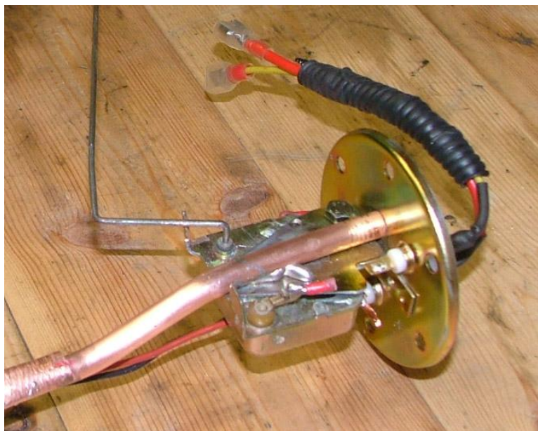
Figure 46 – Electrical module fixed onto the back plate
