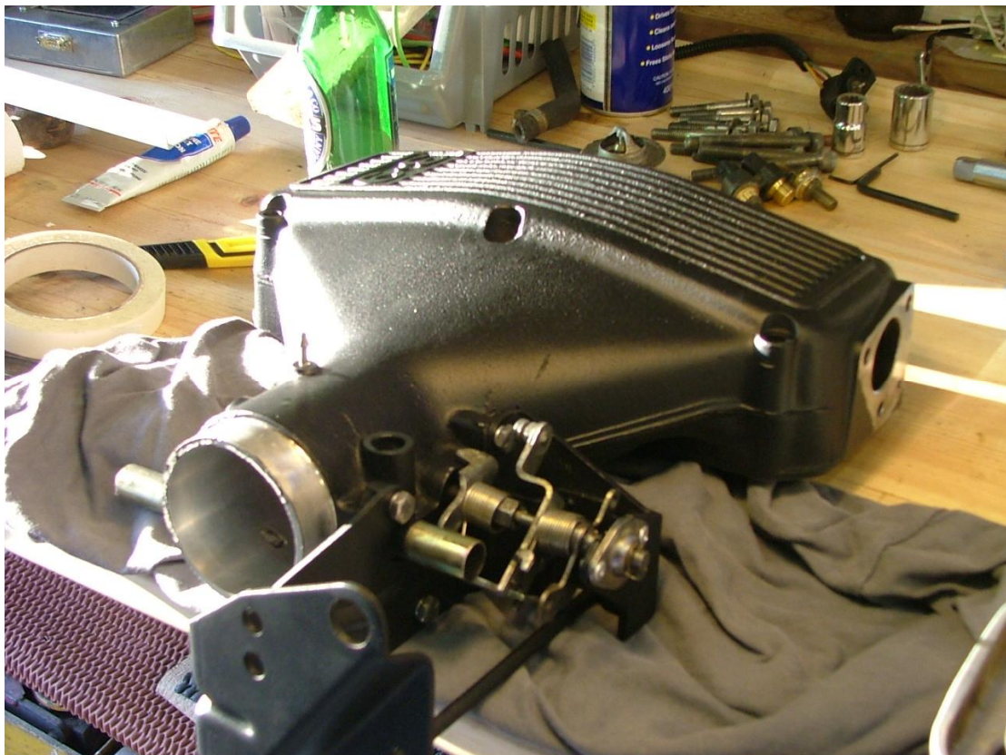
Figure 12 – Sprayed plenum complete with rebuilt throttle linkages
