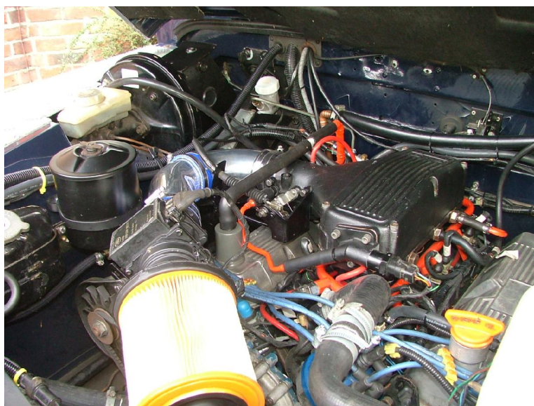
Figure 28 – Mounted air filter (outer canister removed) clipped to MAFS
