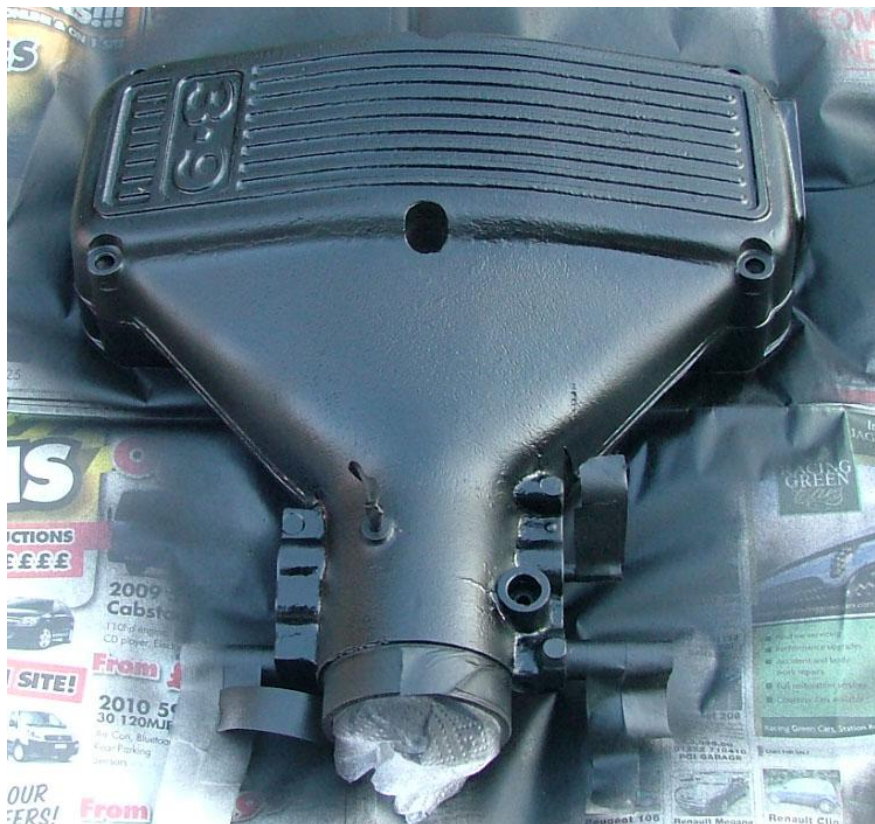
Figure 10 – Painted plenum - minus all ancillary components
