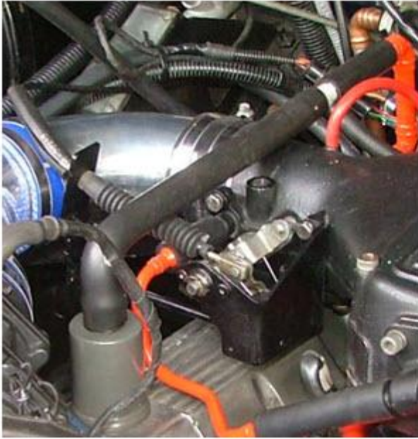
Figure 33 – View of the PCV system pipe routing
