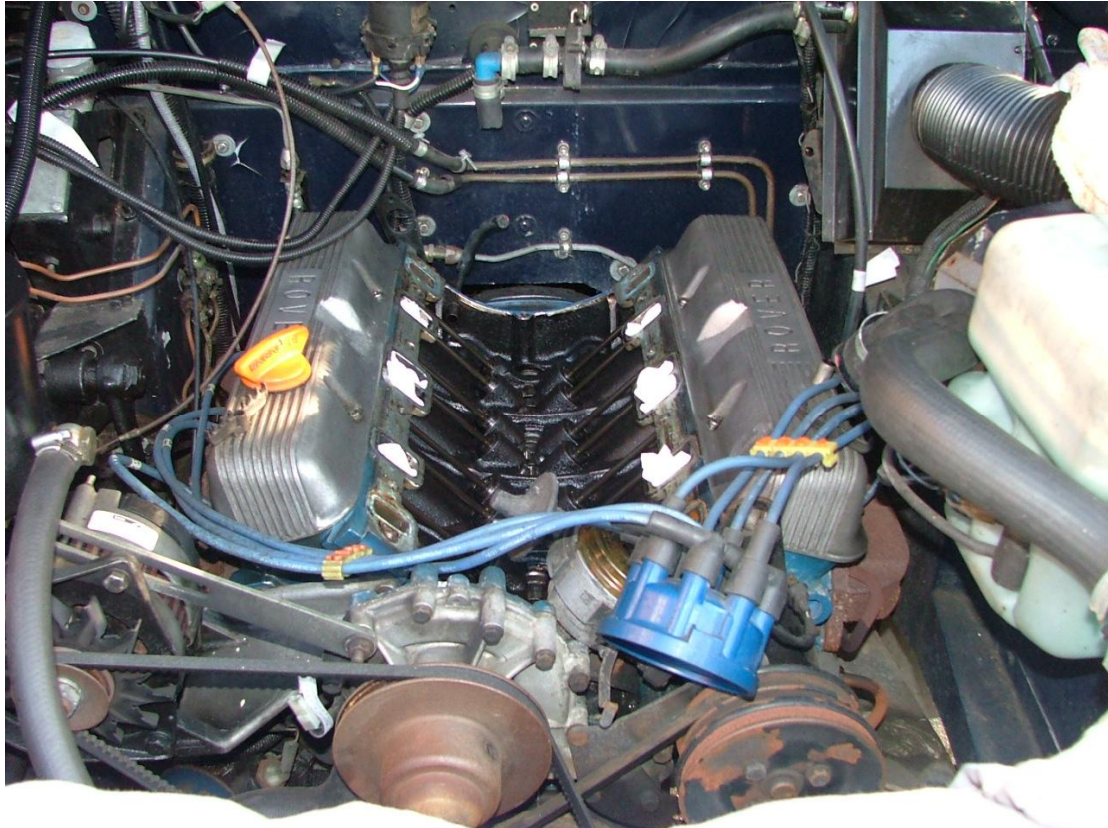
Figure 13 – Rover V8 cleared down to the valley
