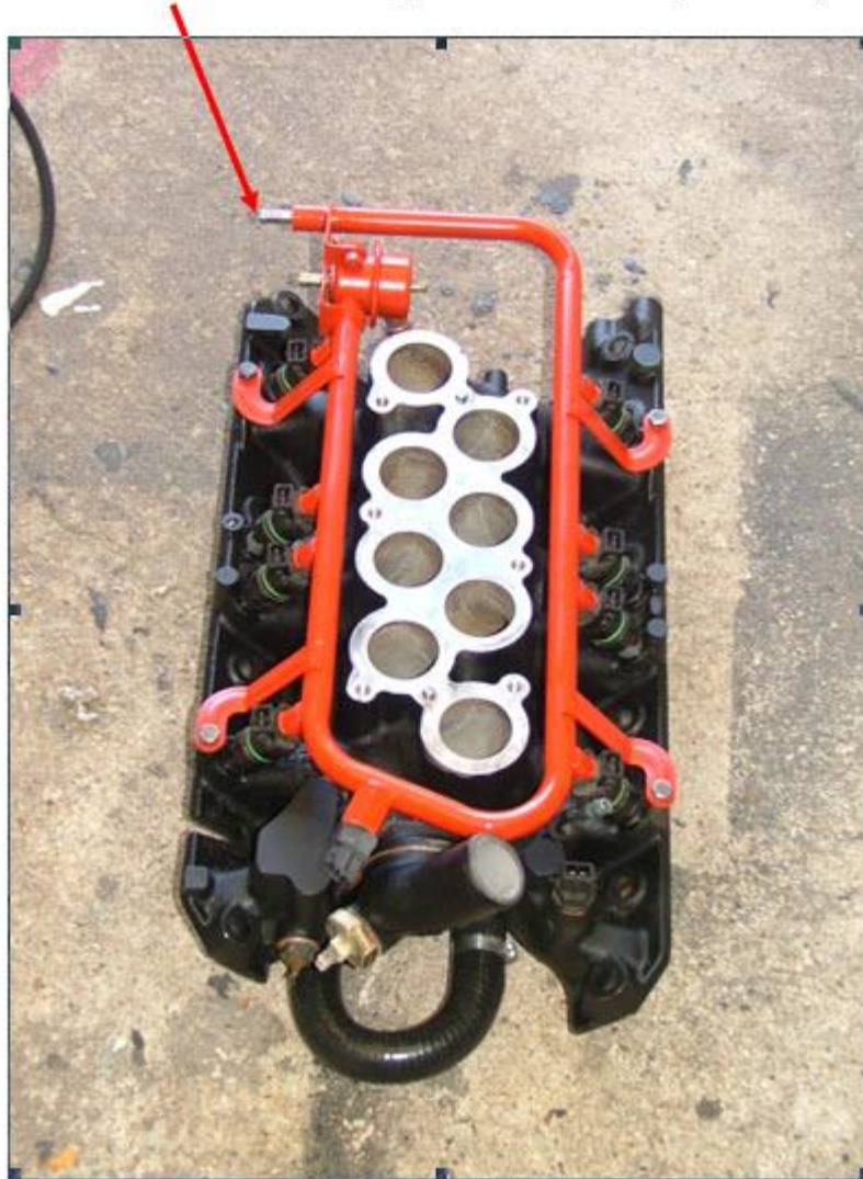
Figure 20 – Finalised injection intake base
