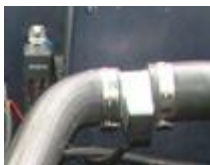
Figure 48 – Digital radiator fan sensor in top hose (control relay behind)
