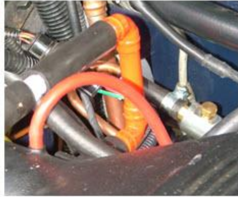
Figure 33 – View of the PCV system pipe routing
