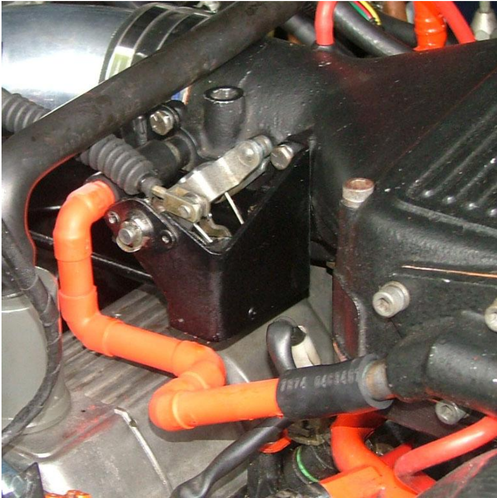
Figure 51 – Idle air supply pipe (red) – finalised
