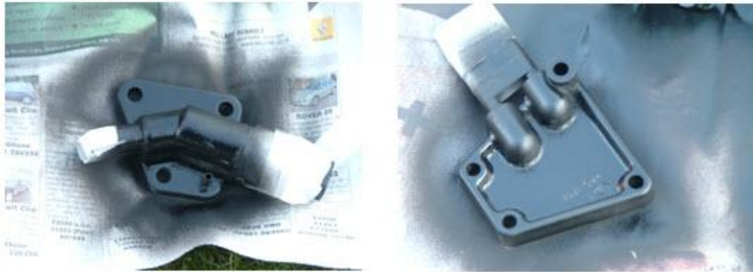
Figure 11 – Sprayed idle bypass air valve housing and plenum pre-heater
