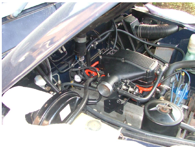
Figure 22 – Final position of the plenum
