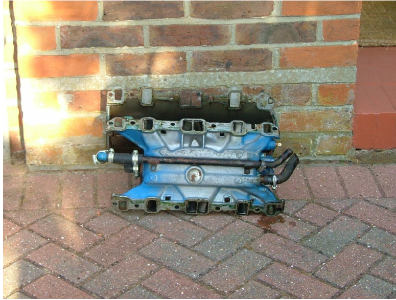
Figure 15 – Underside of original carburettor manifold (showing the plumbing)
