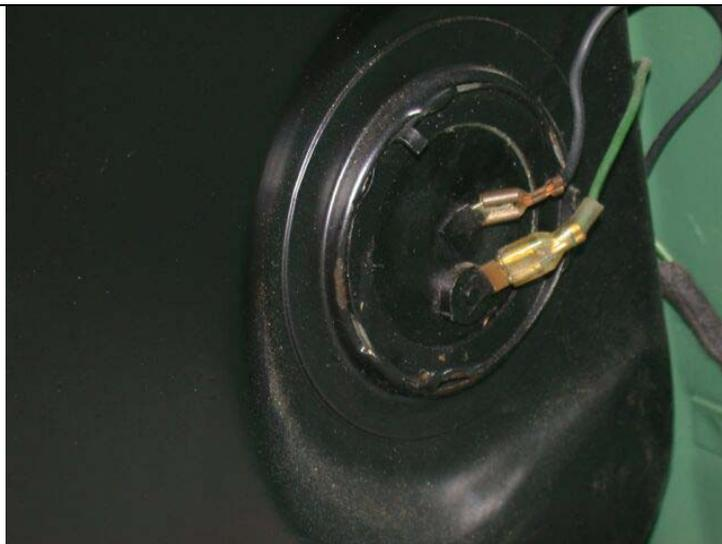
Fuel sending unit wires connections at the tank.
