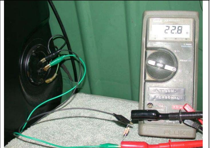
Shown between the two test leads is the additional resistor parallel to the sending unit. The resistor shown here has an actual value of 135 Ohms and as can be seen, this causes the sending unit to appear to have an EMPTY value of near 90 Ohms.
