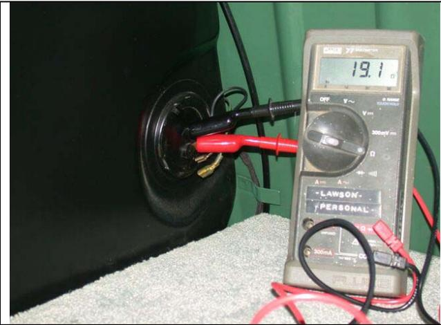
With the float arm pushed down (Empty) and the volt/ohm meter connected, a resistance of about 250 Ohms is measured.
