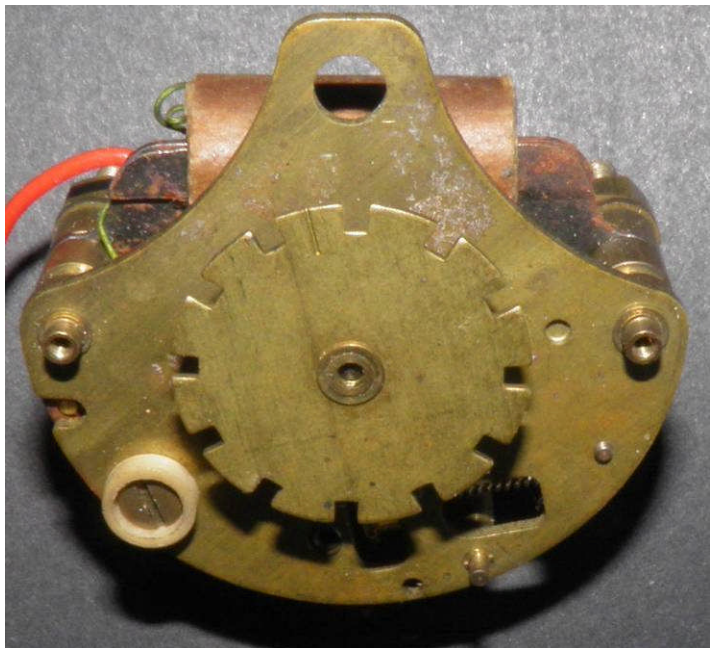
FIGURE A.2: Showing the slotted-disc connector between the clock mechanism and the dial assembly of the (American) Jaeger clock. Connection between the two assemblies was by means of a pin on a crank fitted to the dial assembly that entered one of the slots on the disc seen here.
