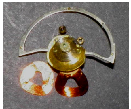
FIGURE 6.2: Damaged balance wheel assembly as removed from Smiths CTE clock.
