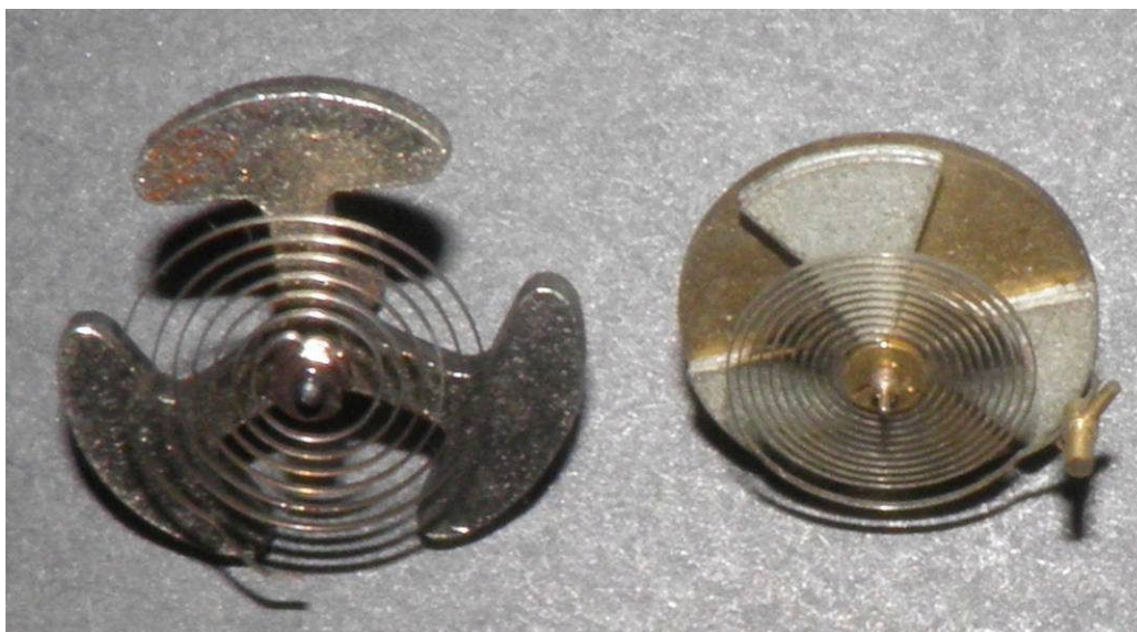
FIGURE A.3: Showing the balance assembly from an American Jaeger clock on the left and that from a Smiths/Jaeger "CE" clock on the right.
