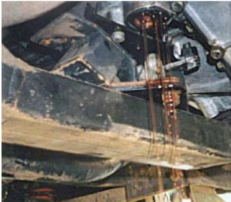
Here the old ATF fluid can be seen draining from the extension case on an LT77 gearbox. Note its characteristic red colour and very thin viscosity
