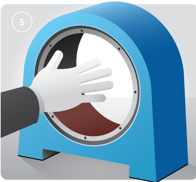
6. Remove the roller assembly from the outer ring prior to assembling the outer ring in the housing. The roller-retainer assembly and outer ring are matched and the roller-retainer must be kept together during mounting process. Place the bearing outer ring (without the roller assembly) into the housing and slide it into place. The outer ring is typically a loose fit and easily mounts in the housing. If needed, use
