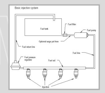
The fuel injector is an electrically-controlled solenoid that allows pulses of fuel to be injected into the inlet ports. The amount of fuel injected is varied by changing the time the injector is open by means of the injector pulse width. There is one injector for each cylinder, and the fuel is kept at a constant pressure differential between the fuel rail and the inlet by the fuel pressure regulator, fitted at the rear of the fuel rail on the left of the engine.
